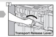
Removing a Misfed Paper (Paper Exit/Fuser Area)
